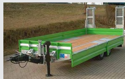
Transporter for construction machinery 6,9 to.
